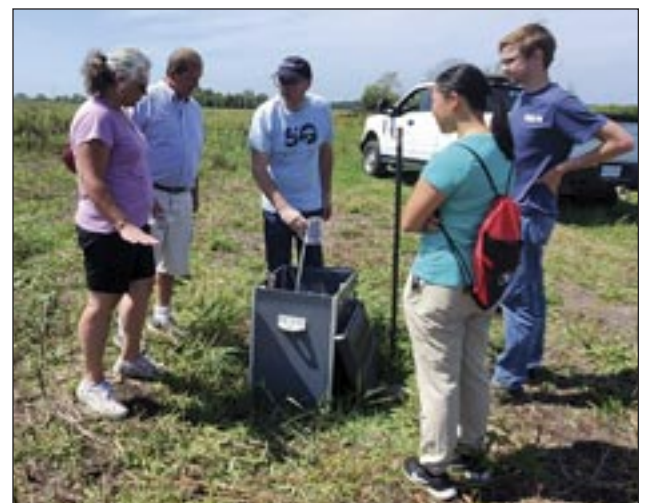
Mike Evans demonstrates how volunteers can take water samples from a woodchip bioreactor. Samples are frozen until they can be tested in a Champaign lab. Photo by Raelynn Parmely.
