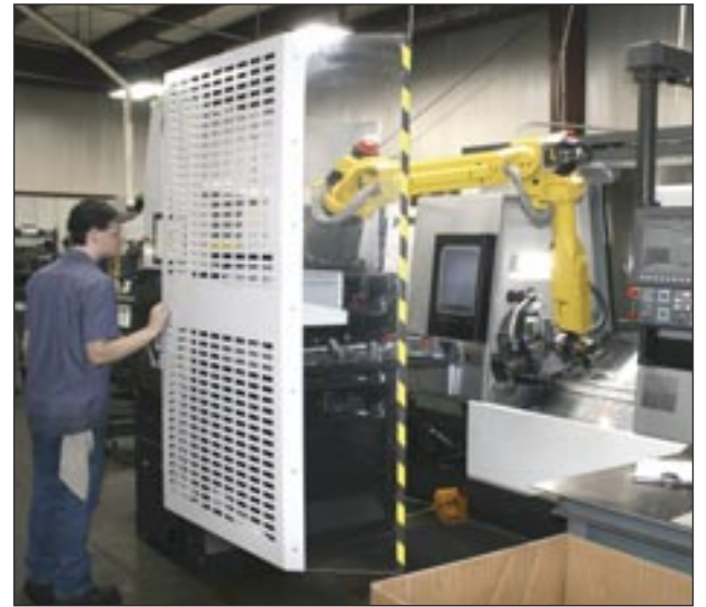
This is a Live tool, sub spindle lathe with a robotic loading system for manufacturing precision parts. Photo by John A. Ballentine..
