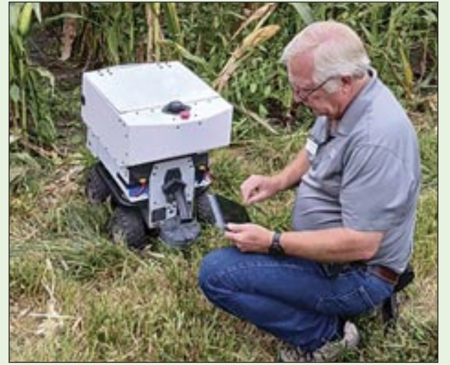
Dennis Bowman works to program a robot planter used to sow cover-crop seeds in rows of standing corn. Photo by Nick Vlahos.
