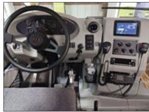
The console of one of Williamsfield’s electric buses includes a screen with details on how much charge is left in the vehicle. Photo by Nick Vlahos.
