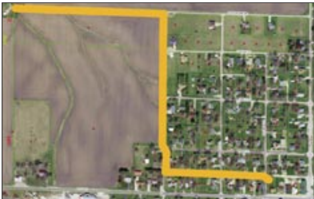
Water used to flush anew well in Yates City will be pumped via hose north and west of town as shown above in yellow.
